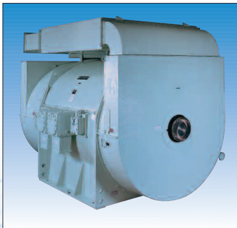
HP compressor drive, Exd IIA T3, 10,000 kW, 11 kV, 4-pole. Low-noise design with absorber and air outlet silencers.
