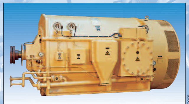
Drive for pipeline oil pump, Exd(e) IIA T3, 2, 600 kW, 6 kV, 2-pole; bearings with force-feed lubrication
